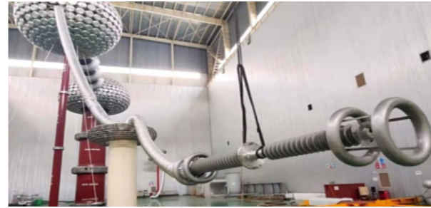
550kV 穿墙套管出厂试验 Routine test of 550kV wall bushing
