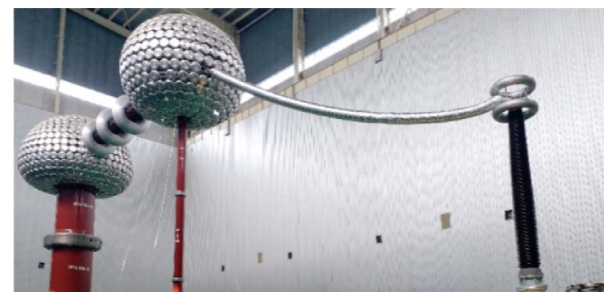
±500kV GIS 出线套管出厂试验 Routine test of ±500kV GIS bushing
