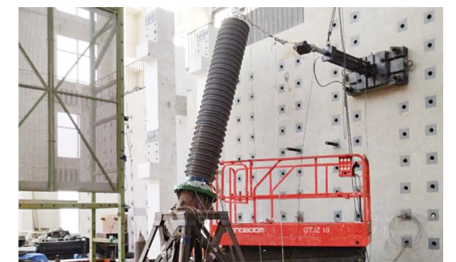
252kV 变压器套管通过了 0.76g 水平加速度、0.62g 垂直加速度的正弦共振拍波地震考核试验 The 252kV transformer bushing passed the sine resonance beat wave seismic assessment test with 0.76g horizontal acceleration and 0.62g vertical acceleration
