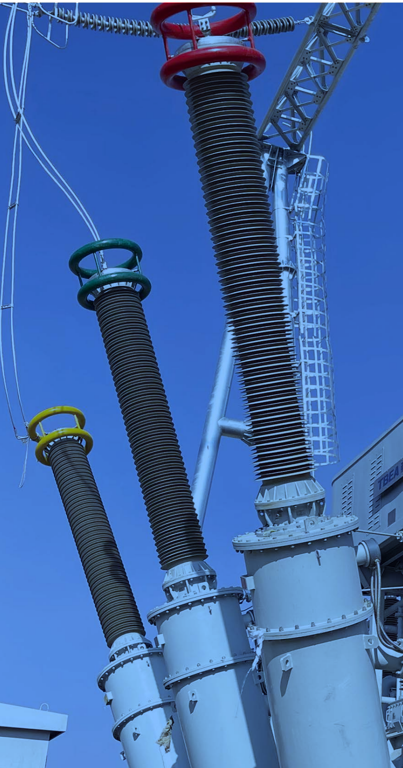
550kV 穿墙套管出厂试验 Routine test of 550kV wall bushing
