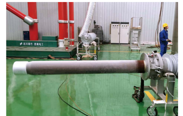
-196°C ~ 室温环境 12 次冷热冲击试验 12 times cold and hot impact tests from -196 °C to room temperature
